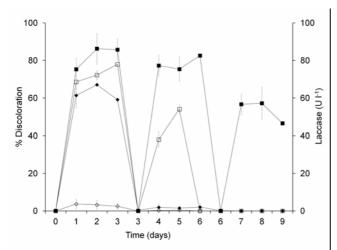
FIGURE 5 - Operative cycles: Percent discoloration with treatments with saturated fiber ( $\blacksquare$ ), Laccase (U L<sup>-1</sup>) with treatments with saturated fiber ( $\ominus$ ), Percent discoloration with treatments with non-saturated fiber ( $\Box$ ), Laccase (U L<sup>-1</sup>) with treatments with non-saturated fiber ( $\ominus$ ).
