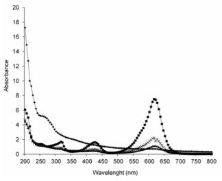
FIGURE 6 - UV/VIS scans of cycles for saturated fiber and 50 ppm of dye: Initial sample ( $\blacksquare$ ), cycle 1 ( $\blacklozenge$ ), cycle 2 ( $\blacktriangle$ ), and cycle 3 (x).
