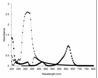
FIGURE 4 - UV/VIS scans of the optimal treatments obtained in the selection of the configuration of the biocarrier, and the effect of the addition of glucose as co-substrate on the dye removal: Initial sample ( $\blacksquare$ ), Treatment 8 ( $\blacklozenge$ ), Treatment 11( $\blacktriangle$ ).
