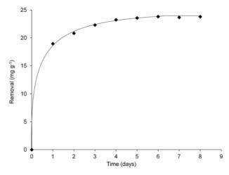
FIGURE 1 - Effect of contact time on Basic Green 4 adsorption to *Agave tequilana* fiber at 25 °C.
