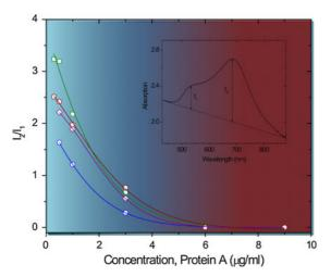
**Fig. 6** Dependence of the ratio  $I_2/I_1$  on the concentration of protein A. The particle sizes of the colloidal solutions used were 16, 18, 20, and 33 nm, according to the order cited in Fig. 1
