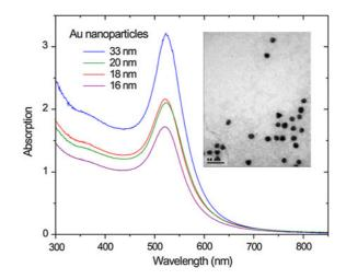
Fig. 1 UV–Visible spectra of the group of colloidal solutions with different concentrations and particle size used in this study. *Inset* TEM image of gold nanoparticles analyzed in this study. For this case d = 15.4 (TEM) and d = 16 nm (theoretical model)
