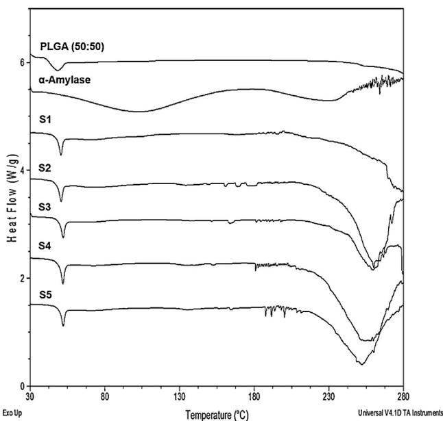
Fig. 6. Differential scanning calorimetric studies. DSC thermograms: from top to bottom; pure PLGA (50:50); pure  $\alpha$ -amylase; S1: system assembled without nanoparticle infiltration; S2–S5: systems with infiltration of nanoparticle suspensions with 25, 50, 75 and 100 mg/mL, respectively. NP's = polymeric nanoparticles.
