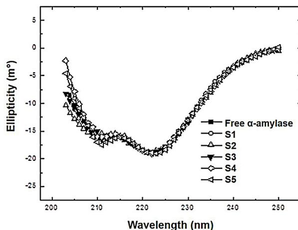
**Fig. 11.** Far-UV CD spectra of  $\alpha$ -amylase after different treatments. Spectra were recorded in 20 mM of phosphates buffer (pH 7.2), at 37 °C. S1: system assembled without nanoparticle infiltration; S2–S5: systems with infiltration of nanoparticle suspensions with 25, 50, 75 and 100 mg/mL, respectively. NP's = polymeric nanoparticles.
