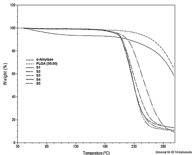
Fig. 7. Thermogravimetric analysis. TGA thermograms: from top to down;  $\alpha$ -amylase pure; PLGA (50:50) pure; S1: system assembled without nanoparticle infiltration; S2–S5: systems with infiltration of nanoparticle suspensions with 25, 50, 75 and 100 mg/mL, respectively. NP's = polymeric nanoparticles.
