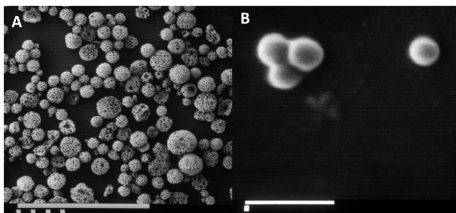
**Fig. 1.** Scanning electron micrograph of (A) porous polymeric microspheres of PLGA 50:50 (scale bar = 1000  $\mu$ m) and (B) polymeric nanoparticles of PLGA 50:50 (scale bar = 1  $\mu$ m).
