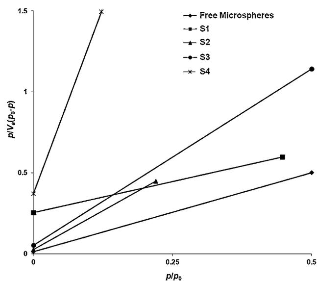
**Fig. 5.**  $\text{N}_2$  isotherms: from top to bottom; (◆) free microspheres of PLGA (50:50); (■) S1: system without nanoparticle infiltration; (▲) S2: system with 25 mg/mL of NP's; (●) S3: system with 50 mg/mL of NP's and (✕) S4: system with 75 mg/mL NP's = polymeric nanoparticles.
