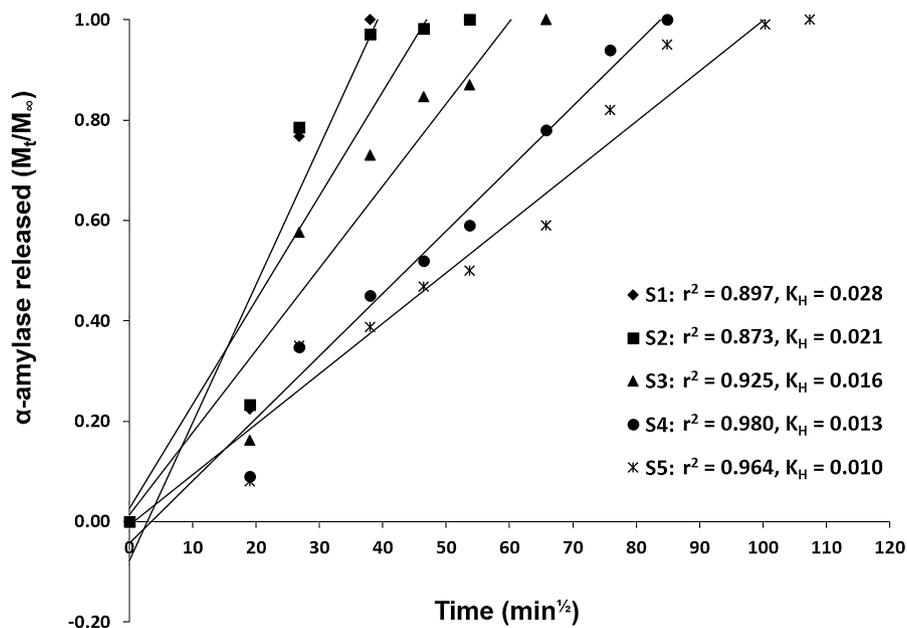
**Fig. 9.** Fit of the release profiles of  $\alpha$ -amylase to the Higuchi's model. (◆) S1: system without nanoparticles infiltration; (■) S2: system with 25 mg/mL of NP's; (▲) S3: system with 50 mg/mL of NP's; (●) S4: system with 75 mg/mL of NP's and (✱) S5: system with 100 mg/mL of NP's. NP's = polymeric nanoparticles.  $M_t/M_\infty$  = amount released at time  $t$ / amount total released.  $K_H$  ( $\text{min}^{-1}$ ) = Higuchi dissolution constant.  $r^2$  = coefficient of determination.
