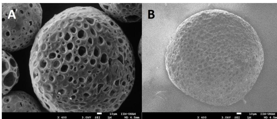
**Fig. 4.** Scanning electron micrograph of polymeric microspheres of PLGA (50:50). (A) free microspheres and (B) microspheres with infiltrated nanoparticles. (Scale bar = 10  $\mu\text{m}$ ).
