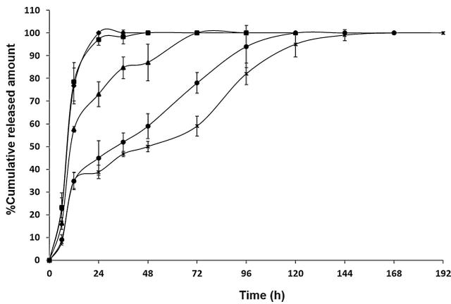
**Fig. 8.** Release profiles of  $\alpha$ -amylase from all assembled systems. Studies performed in phosphates buffer (pH 7.2) at 37 °C. (◆) S1: system without nanoparticles infiltration; (■) S2: system with 25 mg/mL of NP's; (▲) S3: system with 50 mg/mL of NP's; (●) S4: system with 75 mg/mL of NP's and (✱) S5: system with 100 mg/mL of NP's. NP's = polymeric nanoparticles.
